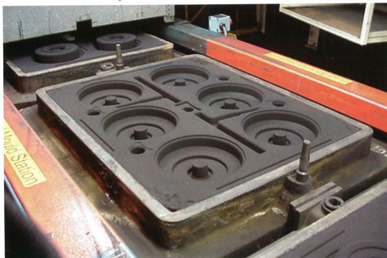
Horizontal greensand moulding line
